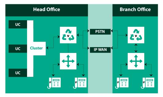
Figure 1. Typical Multisite UC deployment
